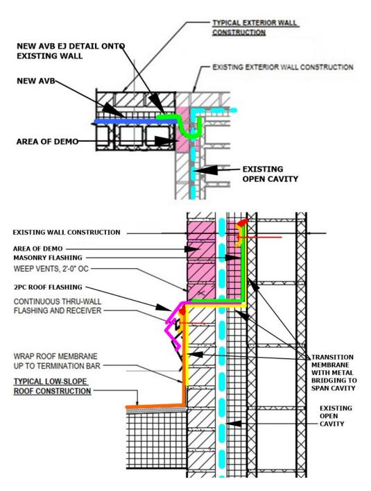
If the existing adjacent building wall construction is a cavity type wall design, the new air/vapor barrier system should close off the wall cavity to prevent exterior air from within the cavity getting into the newly conditioned space. This is even more important in a cold environment where the existing air cavity will likely create condensation within the wall in the newly created interior space.
